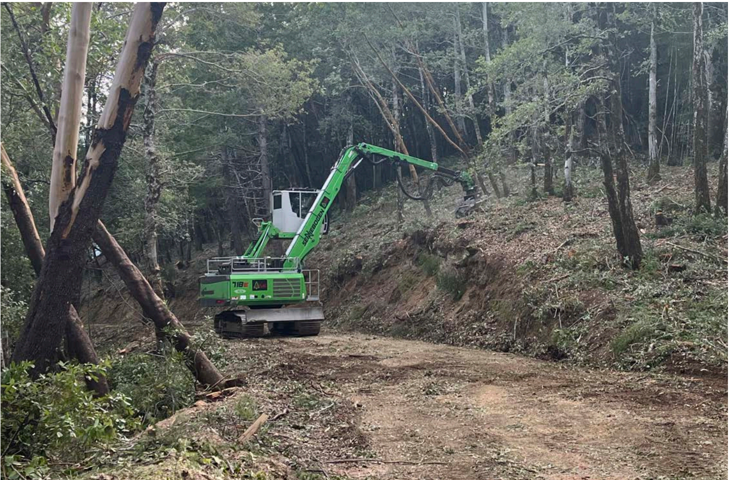
Mendocino RCD: Northern Red Mtn Forest Health Improvement Project, 2023 – Sennebogen 718 E performing roadside fuels reduction
