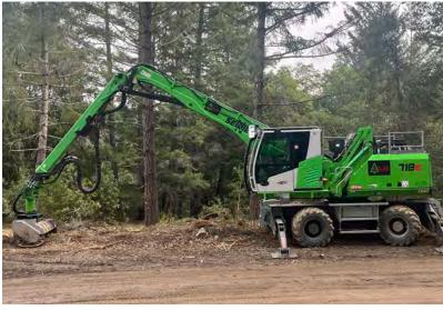
Figure 1. Sennebogen 718 Tree Handler with FAE mastication attachment
