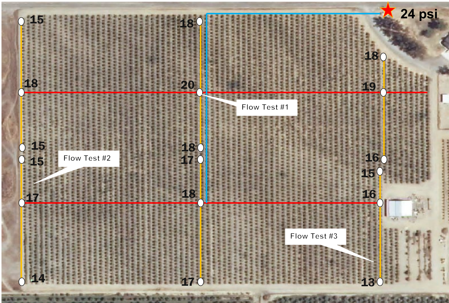
System details – Netafim Supernet Jr. Micros with blue nozzles and 25 psi regulators
